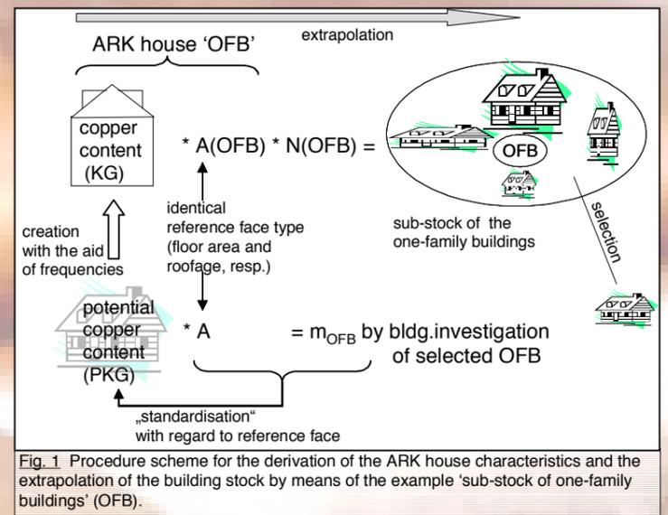
Fig. 1 Procedure scheme for the derivation of the ARK house characteristics and the extrapolation of the building stock by means of the example 'sub-stock of one-family buildings' (OFB).
