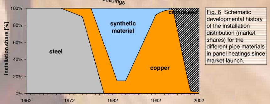
Fig. 6 Schematic developmental history of the installation distribution (market shares) for the different pipe materials in panel heatings since market launch.
