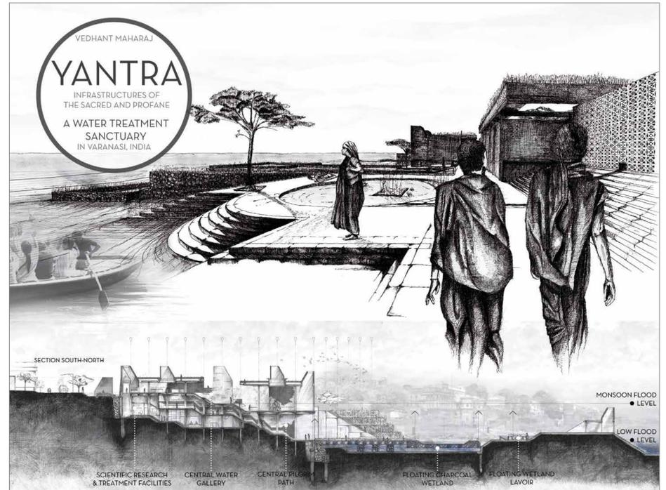
Image 1: Top: Perspective south under high flood conditions. Charcoal gabion walls are submerged. Layered breeze blocks create a ventilated boundary for the female bathhouses on the right of the image. Bottom: East-west section. Scientific research and treatment facilities are located underground. A pilgrim path acts as a direct link to the main floating charcoal wetland pool. The central water gallery cascades along the ground plane. Tall stone turrets ventilate underground facilities.
