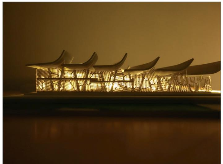
Image 2: Elevation view of screen and roofline at night: A locally sourced bamboo and wood permeable dust filtering screen allows for cross ventilation and passive thermal control of the space, while filtering and emitting a glowing light gained from the roof PV's at night. The section shows the ascending curve in the roof which shields the interior from peak heat while creating clerestories for optimal diffused natural light within.
