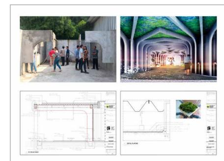
Image 10: Left: 1:1 foamcrete mock-up panels and detail. Right: moss ceiling impression and detail.
