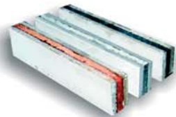
Figure 01 - Sandwich beams for Flexural tests.
