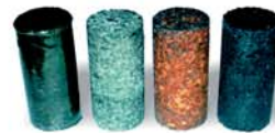
Figure 03 - Composite core materials. Leather shavings PU coated, leather shavings, wood chips, rubber.
