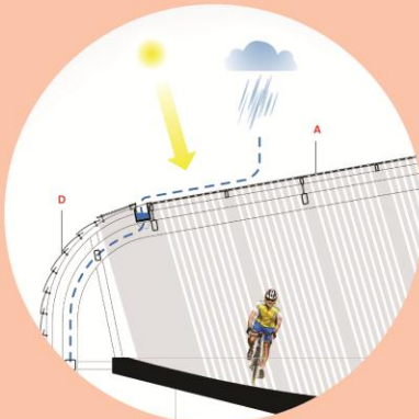
DETAIL AA: PHOTOVOLTAIC PANELS AND RAINWATER COLLECTION
